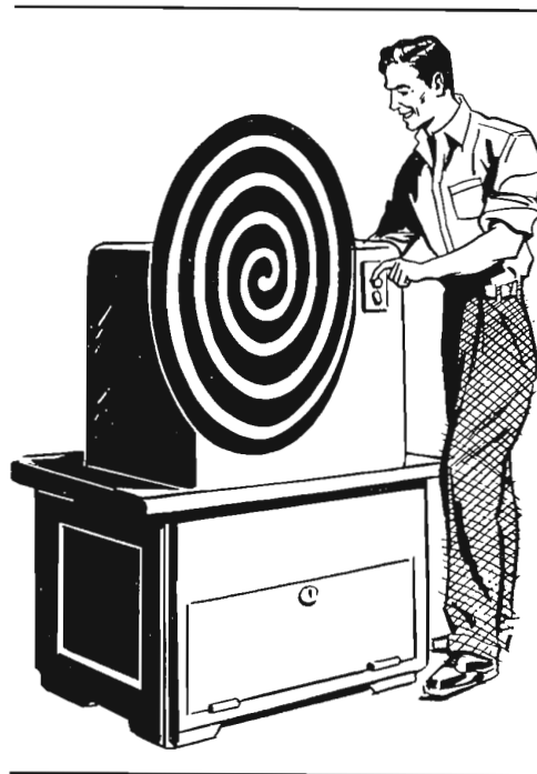
FIG. 25. A studio "transitor" used for special effect and montage shots. The crewman controls the speed of the disc.
